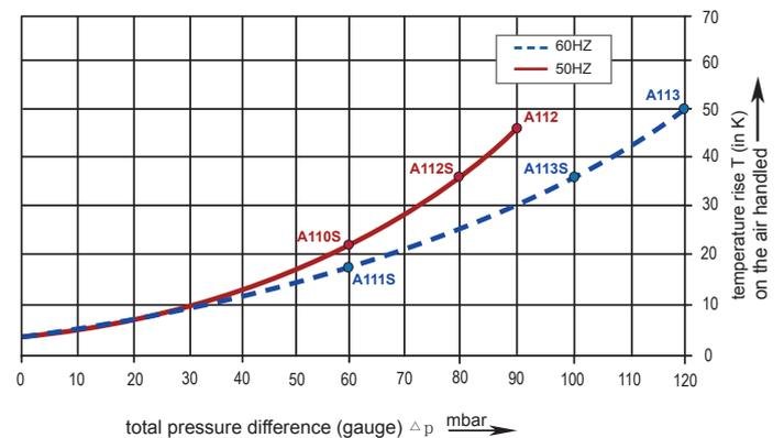
The performance curves are based on air at a temperature of 15 °C and an atmospheric pressure of 1013 mbar with a tolerance of +/- 10 %. The total pressure differences are valid for suction and ambient temperatures up to 25 °C. For other conditions please confer with us.
